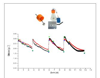
Pic. 7: Comparison of HPLC, off-line analysis and in-situ sensors in a real cell cultures. All methods are optimized for biotechnology applications. All three methods do vary a little from each other but you can't see a clear tendencie to a certain method which is more precise than the others. If you compare three methods you cannot expect higher precission than <10%. In most applications this is far good enough to work with.
