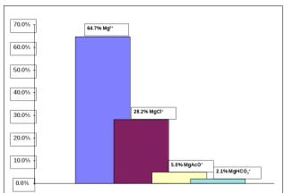
Pic. 2: Different fractions of Magnesiumchlorid when disolved in water. Ion selective sensors do measure only the Mg2+ fraction while AAS (Atomic Absorbtion Spectroscopy) measures the totel concentration. In this example the difference in the result will be around 30%
