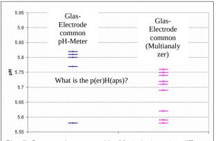
Pic. 7: One sample measured by 22 students on two different pH measuring devices. The difference is up to 0.3 pH units
