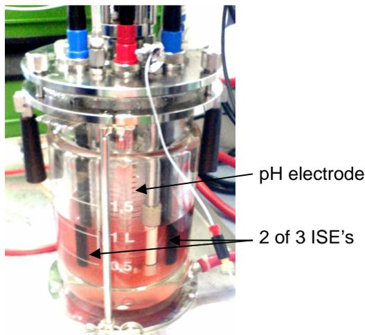
Figure 1: Bioreactor with a pH and two of three ammonium ISE's.
