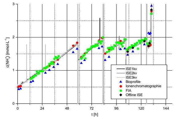
Figure 3: Results of the continuous in-line monitoring and the comparison to on-line and three different off-line analyses.
