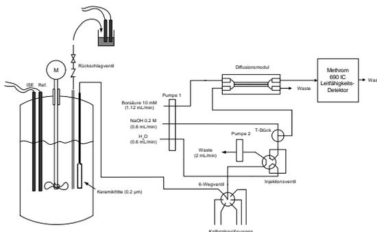
Figure 2: Scheme of the whole set-up.
