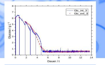
Automated Process Control based on in situ measured Glucose Concentration
